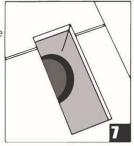
Heating vents require expansion room. First, cut plank to the correct length. Place the cut plank at its actual
