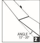
Insert 2nd plank's end tongue to 1st plank's end groove at an angle of 15° to 20°. The plank will click into place when lowered. Line up edges carefully. Planks should be flat to the floor.
