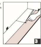
For the last plank of a row, flip a full plank to its under side and place beside the row.
