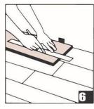
To fit the final row, lay a plank upside down on the flooring as per diagram with the tongue side close to the wall.
