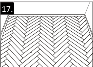
17. Spacers and skirting Remove the spacers and cover the expansion gap with skirting boards or beadings.
